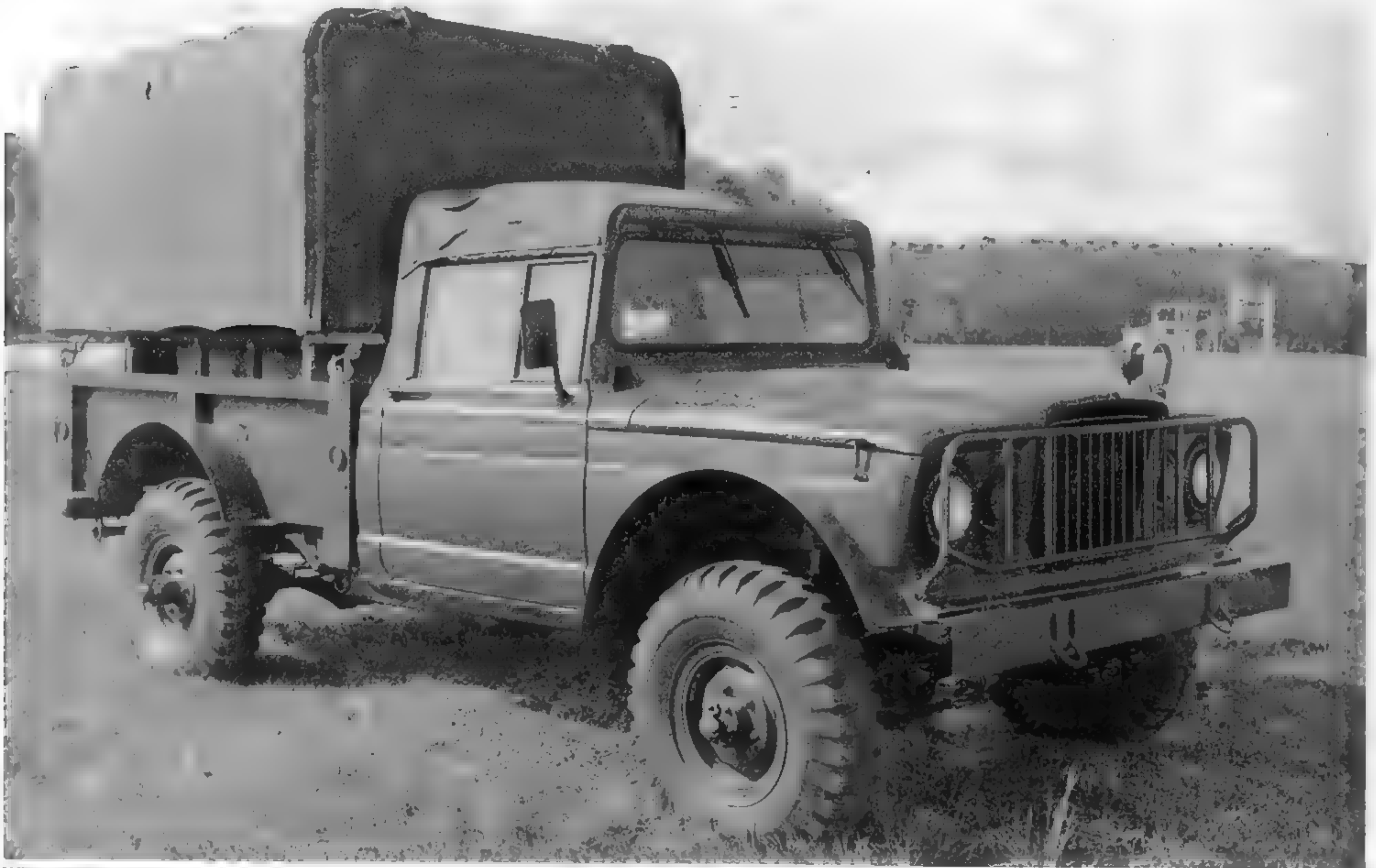
When set up to transport, the S-250 shelter was known as the M142. This truck may well have been the pilot model of the M142. (U.S. Army photo)
